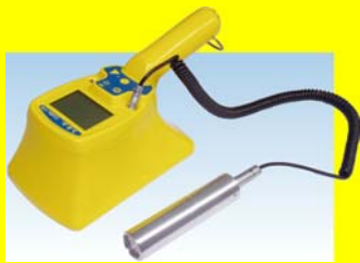
CoMo with connected detector for dose rate measurement
